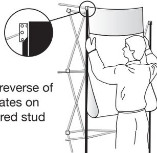
Align panel edges down centre of magnetic bar
